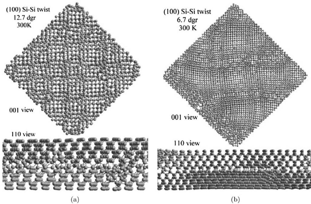
Figure 3. MD simulated structural models ([001] and [110] views) of bonded wafers with different rotationally twist angles annealed at 300 K for parallel dimer start configurations: (a)  $12.7^\circ$ , 6500 atoms, 4.9 nm box; (b)  $6.7^\circ$ , 23000 atoms, 9.2 nm box.
