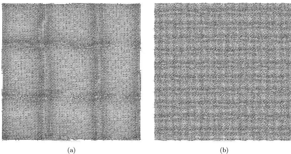
Figure 9. MD-simulation of bonding thin wafers with rotational twist: [001] view of MD relaxed model with  $2.8^\circ$  (a) and  $12.7^\circ$  (b) twist.
