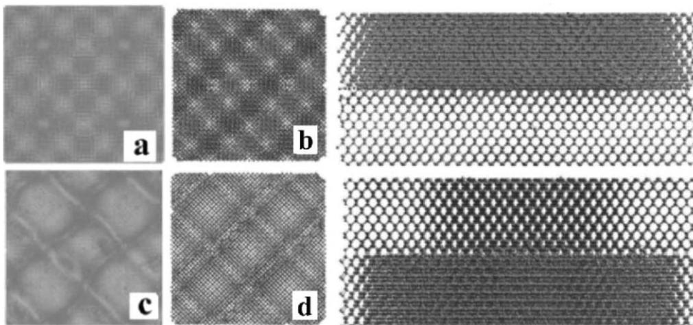
*Figure 5.* MD relaxations of bonding rotationally twisted wafers ([001] views and in addition for (b) and (d) [110] views, resp.) with different angles: (a) 2.8°, 134500 atoms, 22 nm box, orthogonal dimers, (b) 6.7°, 9.2 nm box, orthogonal dimers in start, i.e. an additional 90° twist; (c) as (a) and (d) as (b) with parallel dimer start configuration.
