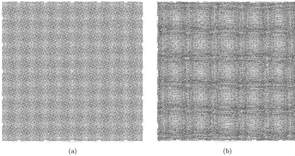
Figure 7. Simulation of thin bonded wafers with  $6.7^\circ$  rotational twist: [001] view of initial (a) and MD-relaxed (b) model showing the resulting screw network.
