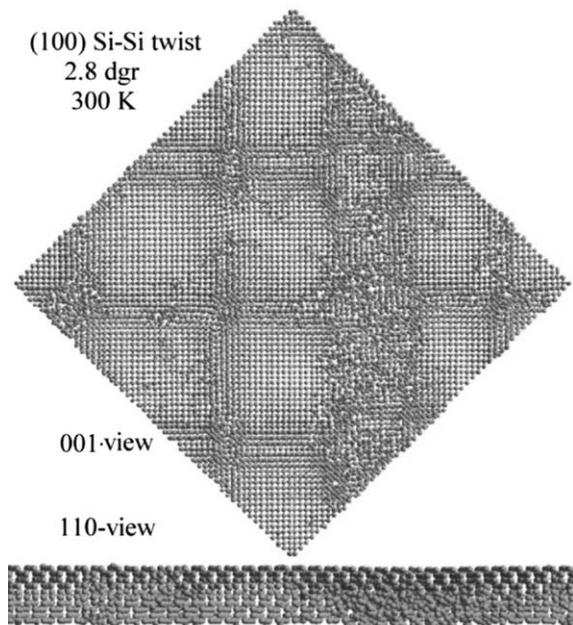
Figure 4. MD simulated structural model ([001] and [110] view) of bonded wafers with a  $2.8^\circ$  rotationally twist angle annealed at 300 K for parallel dimer start configurations: 134500 atoms, 22 nm box with additional bonding over steps along [110] indicated by the broad band at the right.
