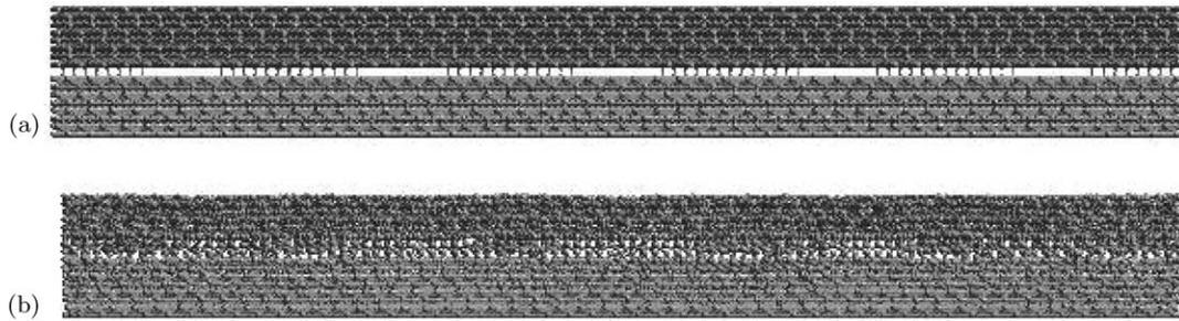
Figure 8. Simulation of thin bonded wafers with  $6.7^\circ$  rotational twist: [110] projections of initial (a) and MD-relaxed (b) model showing bonding details at the interface.
