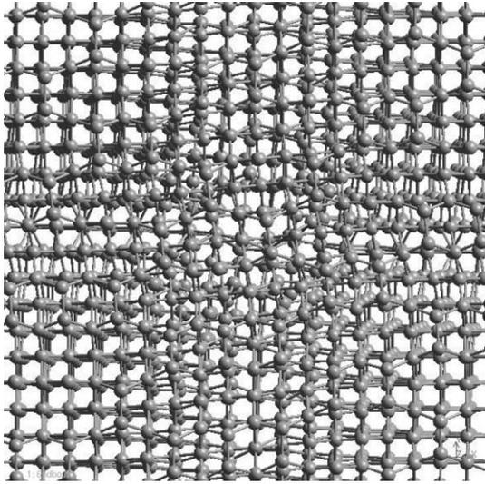
Figure 10. A typical node of  $[110]$ - and  $[\bar{1}10]$ -screw dislocation intersection of the  $6.7^\circ$  twist bonded interface resulting from MD simulated bonding of thin wafers.
