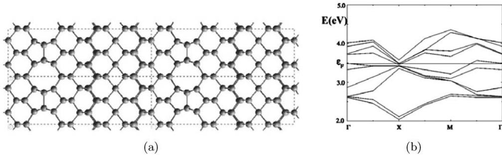
Figure 1. MD simulated structural model (a) of the  $Pmm(m)$  interface at  $90^\circ$  twist and corresponding DFT band structure (b).
