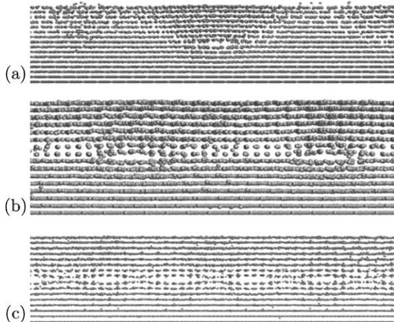
Figure 11. Interfaces after MD-relaxation of thin bonded wafers with  $2.8^\circ$ ,  $6.7^\circ$  and  $12.7^\circ$  twist (a,b,c) in  $[110]$  projection showing the different defect core structures.
