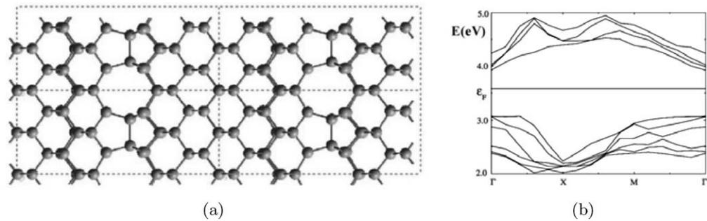
Figure 2. MD simulated structural model (a) of the  $P(\bar{4})m2$  interface at  $90^\circ$  twist and corresponding DFT band structure (b); The dreidl structure reduces the interface energy by approximately 20%.
