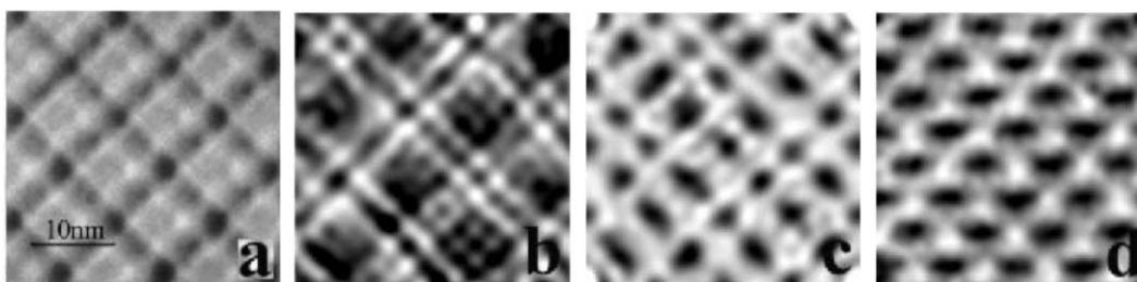
*Figure 6.* Experimental 400kV bright-field diffraction contrast (a) of a 2.4°-twist bonded interface (Courtesy: R. Scholz, MPI-Halle) and simulated TEM images (b-d, 400kV, thickness  $t \sim 40$  nm, varying beam tilt) of models as b and d from Fig. 5: (b) parallel dimers in start configurations, 4.6°-twist, 13.5 nm box, (c,d) orthogonal dimers in start configuration, 6.7°-twist, beam along zone axis and tilt into [200]-excitation, respectively.
