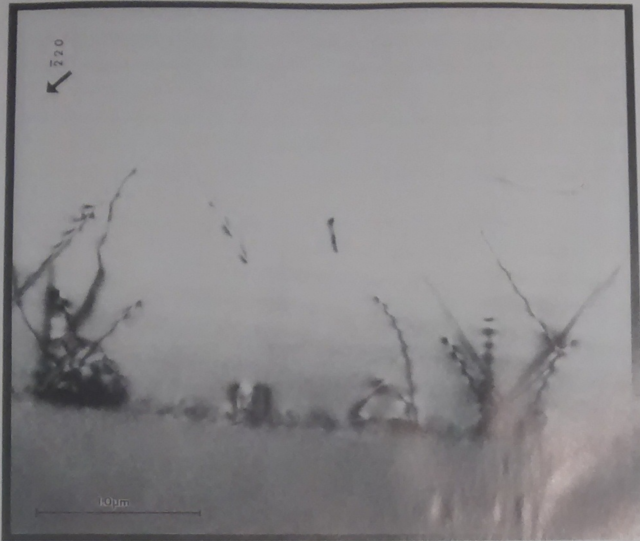
Fig. 2. Electron diffraction contrast image showing high density of defects in GaAs.
