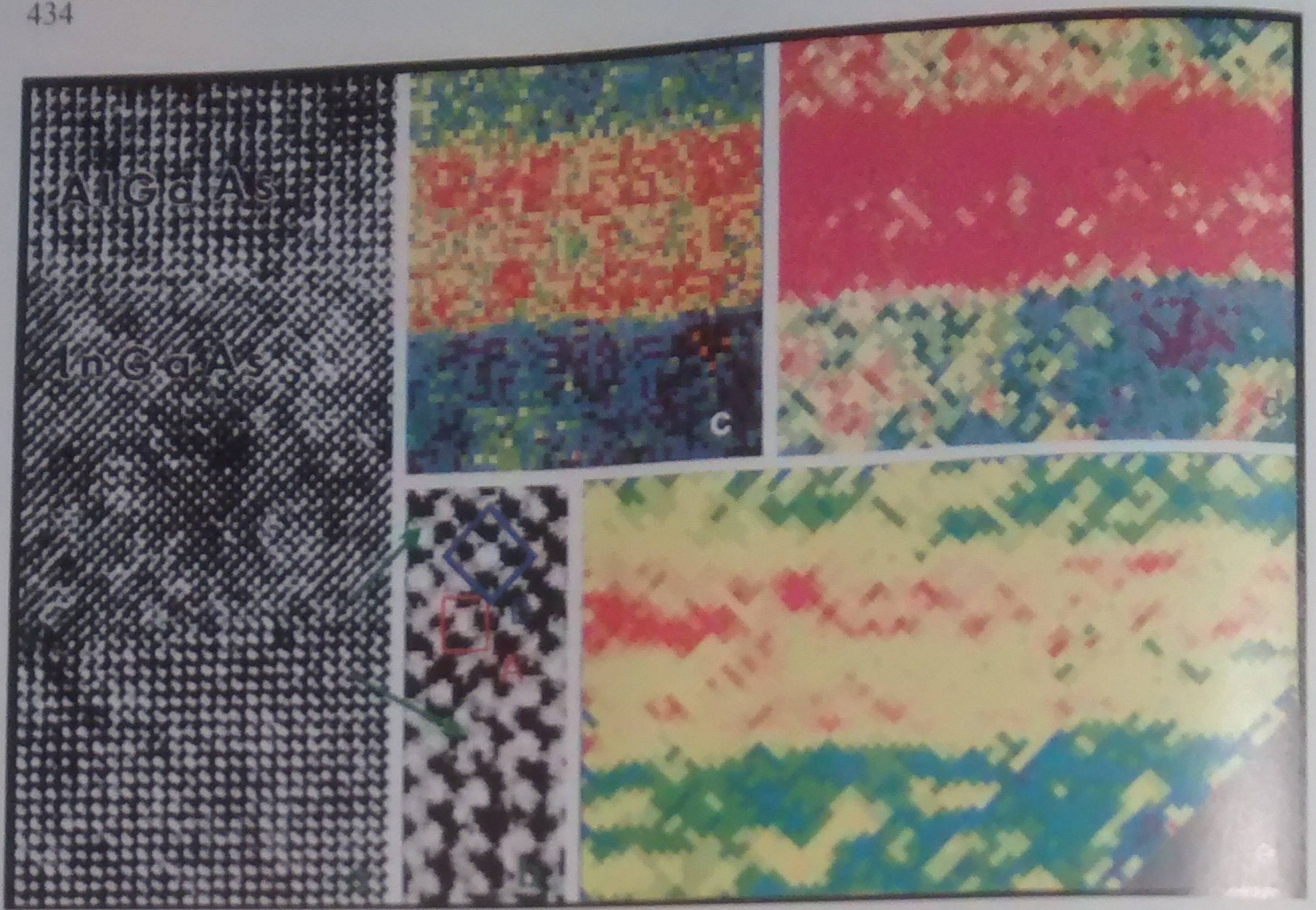
Fig. 6. a) \langle 100 \rangle HRTEM image of test structure T5 with the lower interface partly enlarged (b) showing the two different image unit cells "A" and "B", which are used for chemical mapping ("A" in Fig. 6c and "B" in Fig. 6d). c) The strain mapping with image unit cells of type B
