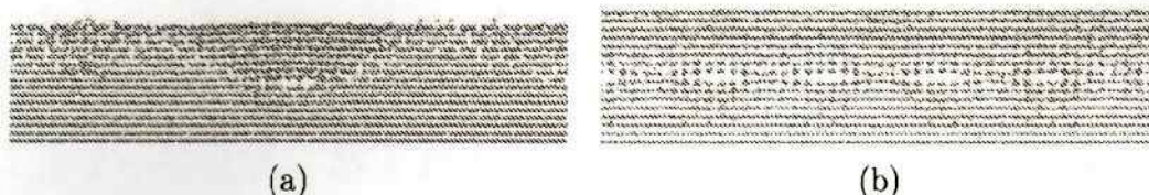
Figure 8: Interfaces after MD-relaxation of thin bonded wafers with 2.8° (a) and 12.7° twist (b) in [110] projection showing the different defect core structures.
