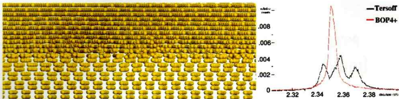
Fig. 6. MD relaxation of bonding rotationally twisted wafers with 8.8^\circ angle, 11 nm box, orthogonal dimers: (a) Interface region in approximately [100] view of the lower crystal part, (b) pair distribution of five adjacent layers around the interface.
