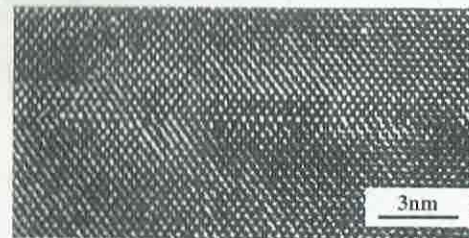
Fig.5: Cross-sectional transmission electron micrograph of the interface of two (100) silicon wafers bonded at room temperature in UHV
