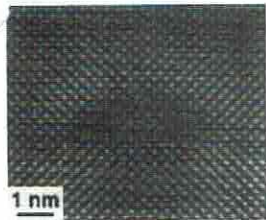
Fig. 4. Simulated HREM image of pyramidal InAs QD in GaAs (400 kV, C_s=1 mm, a_0=0.6 \text{ \AA}^{-1} , def=-70 nm, foil thickness t=22.6 nm).
